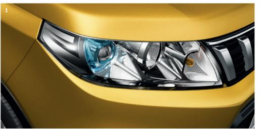
**LED headlamps 1**Bright LED headlamps are used to conserve energy on low-beam. The blue-coloured projector creates a cool impression.
